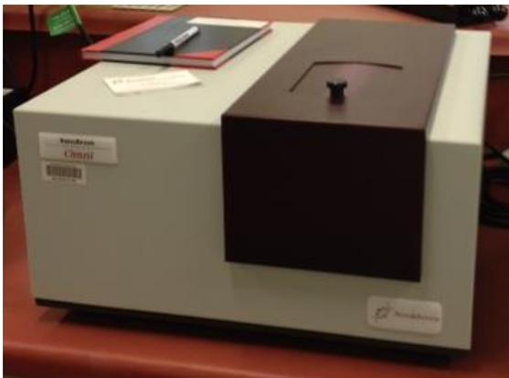
Brookhaven's NanoBrook Omni Particle/Protein Size and Zeta Potential Analyser
